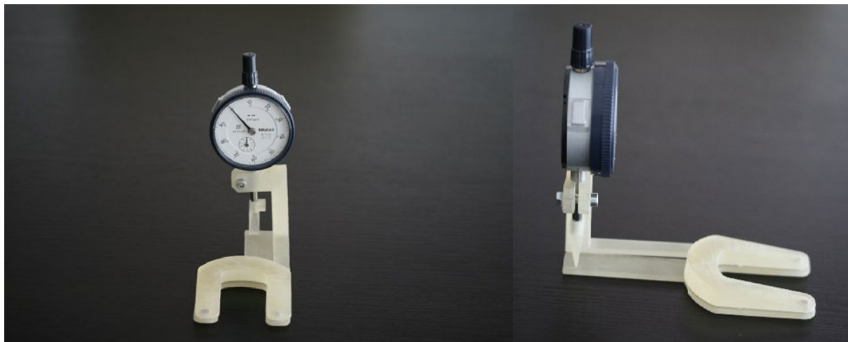
Figure 3. Major components of the Bite Training Machine: dynamometer, force indicator and occlusal area
